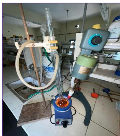
Figure 1: Experimental setup used for the synthesis of Oxazoline
