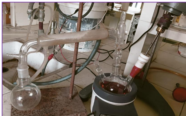
Figure 3: Apparatus used for purification by distillation after synthesis
